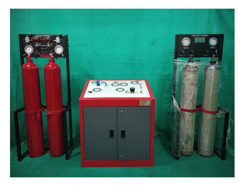
Special gas boosting system is designed for the poisonous gases, flammable gases and mixed gases. Since this system is designed for special gases, it is equipped with gas detector which provides this system well reliable and hi-tech. **Special Gases filling stations** used for filling cylinders of any pressure generally up to 120 bar or higher pressures on request.
