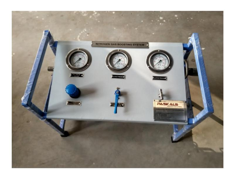
Nitrogen Gas boosting is used to boost the Nitrogen gas from the range of 2500 Psi to 11000 Psi with 6-8 bar drive air at 10-80 scfm flow. This system shall be mounted on suitable Frame Structure in which gas booster, Pressure gauge, pressure regulator, valves and others items shall be present.
