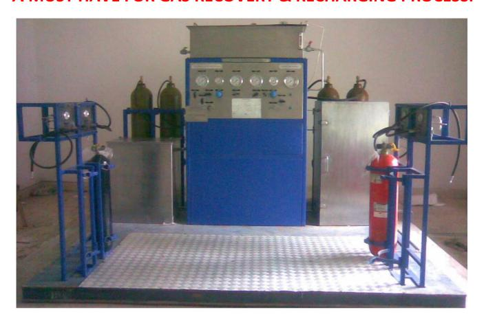
**Helium Decanting System** is a HIGH PRESSURE facility for **Decanting of** the Helium **Flight Bottles** which are accessories to emergency floatation system of the Helicopter.
