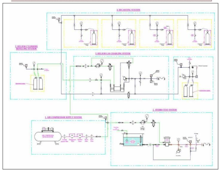
High Pressure HELIUM is recovered and pressurized using Air Driven Gas Booster from Haskel USA (<u>www.haskel.com</u>) up to 400 bar.
