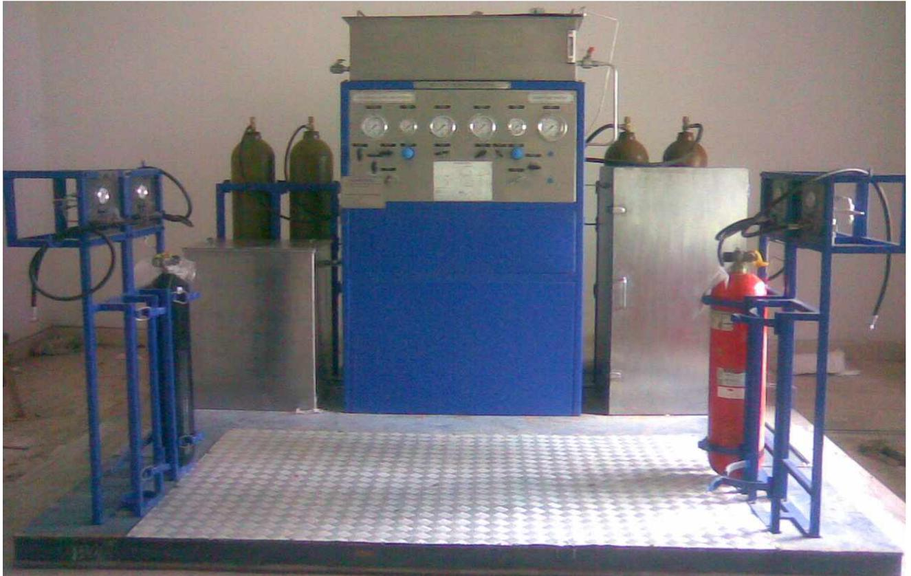
**Helium Re-Charging & Hydrostatic Testing System** is a HIGH PRESSURE facility for **Decanting, Hydrostatic Testing and Refilling** of the Helium **Flight Bottles** which are accessories to emergency floatation system of the Helicopter.
