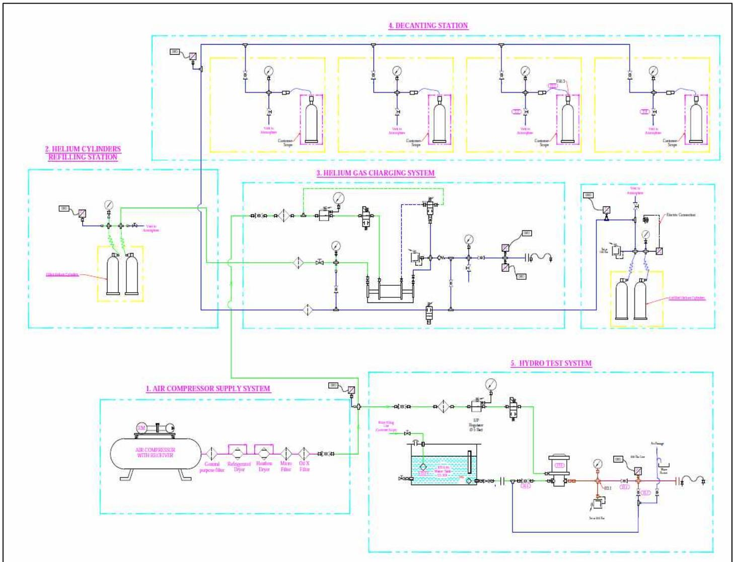
High Pressure HELIUM is recovered and pressurized using Air Driven Gas Booster from Haskel USA ([www.haskel.com](http://www.haskel.com)) up to 400 bar and Hydrostatic Testing at a Pressure of 700 bar using HASKEL USA Make AIR DRIVEN PUMP.
