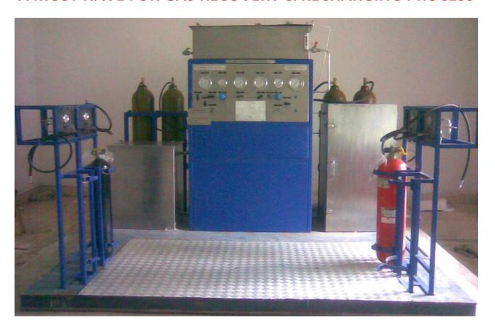
Helium Re-Charging & Hydrostatic Testing System is a HIGH PRESSURE facility for Decanting, Hydrostatic Testing and Refilling of the Helium Flight Bottles which are accessories to emergency floatation system of the Helicopter.
